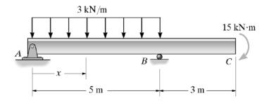
4. Determine the equation of the elastic curve. Specify the deflection at C. EI is constant. 【试 求图示梁的挠曲线和截面 C的挠度。设弯曲刚度 EI 为常数。】
