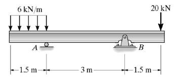
2. The beam is subjected to the load shown. Determine the displacement at x = 7 m and the slope at A. EI is constant. 【试求图示梁在 x = 7 m 处的挠度和截面 A 的转角。设弯曲刚度 EI 为常数。】
